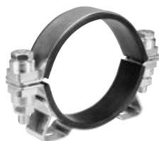
In the NORMACLAMP® HMK two-parts heavy duty version, the ends of the brackets are folded back and spot-welded onto the band.
