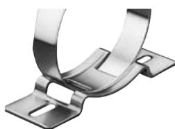
The NORMACLAMP® HMK K1 are prefabricated brackets which you can use to transform NORMACLAMP® standard clamps (types GBS, HD, SP and TORRO) into retaining clamps with brackets in no time at all. Just open the standard clamp, guide the band through the bracket slot, and that's all there is to it.
